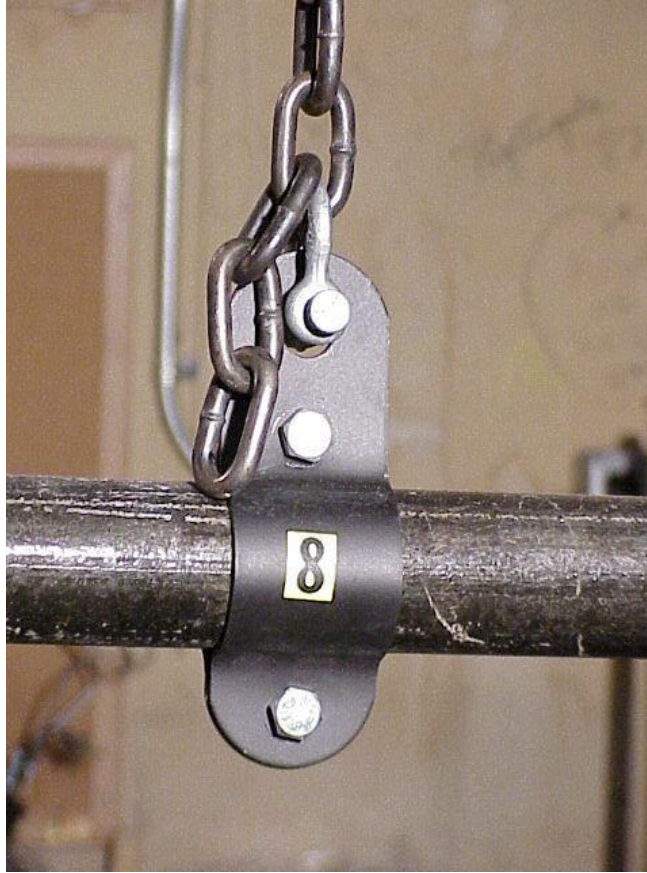
Photo 3 - Showing Trim Chain, Shackle and Batten Clamp
